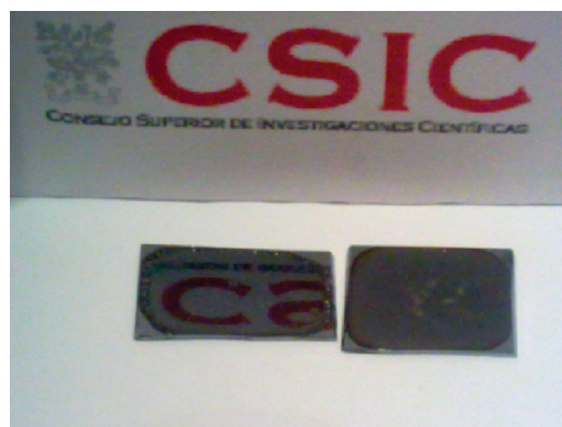
Figure 11. Images of films formed after annealing at 150 °C during 24 h, from PS latex stabilized with 3.2 wt % of PS 40 - b -PPEGMA 70 (left film) and PMMA latex stabilized with 3.2 wt % of PS 40 - b -PPEGMA 70 (right film).
